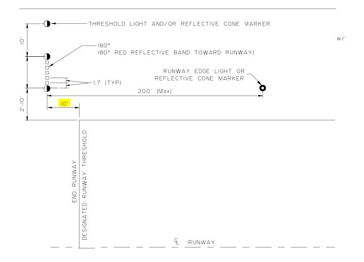
Figure 660-1 Typical Threshold Detail No Scale
