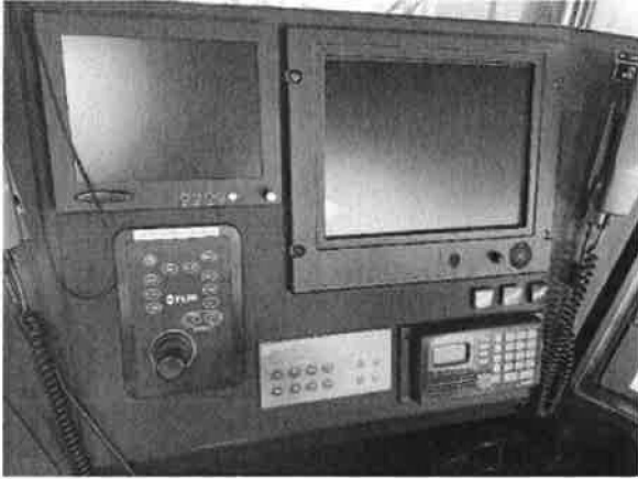
Figure 52 Nauticonning-Raytheon Marine Conning Display and controls in Pilothouse
