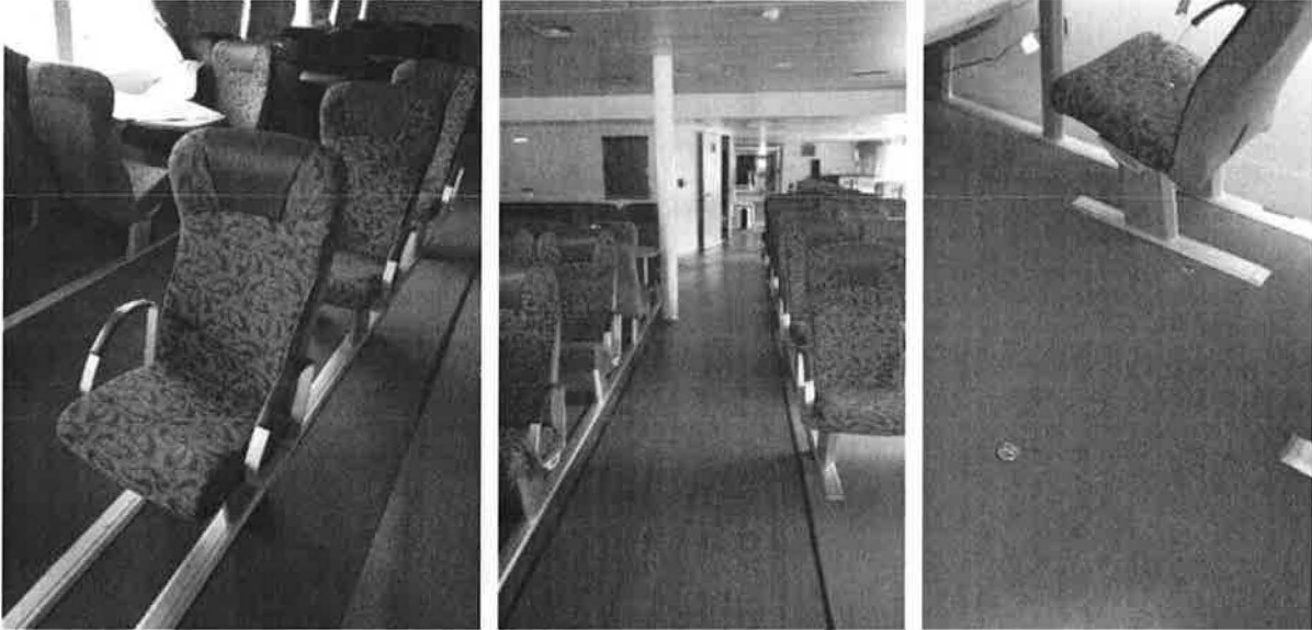
Figure 9 Replacement seats (left), replacement faux wood flooring (middle), and replacement carpet (right) in Forward Observation Lounge
