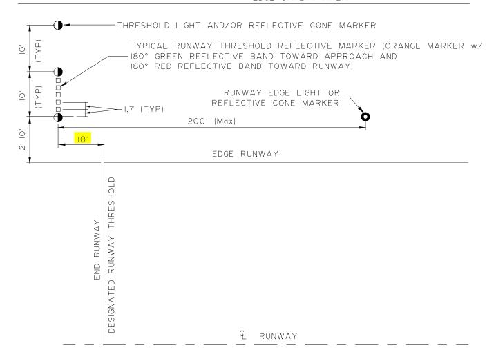
Figure 660-1 Typical Threshold Detail No Scale
