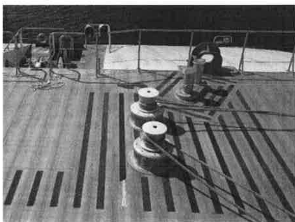
Figure 29 Mooring capstans and fairlead on Forward Mooring Deck
