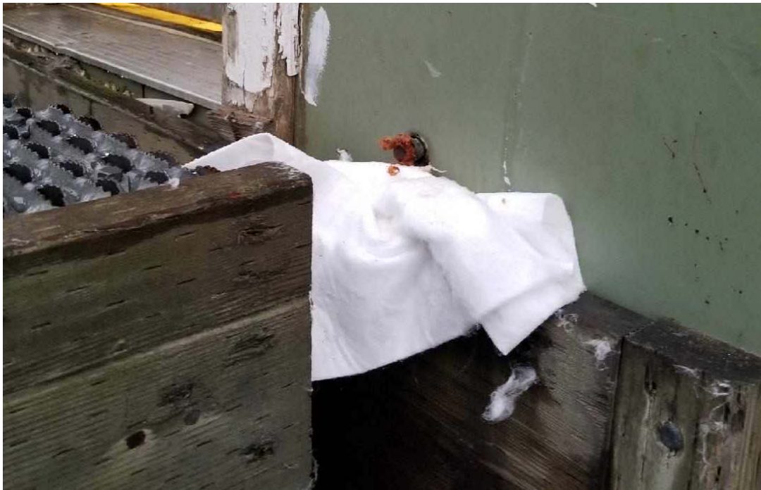
Wooden plug in sheared-off end of line where spill originated from; white absorbent pad placed underneath to absorb fuel.
