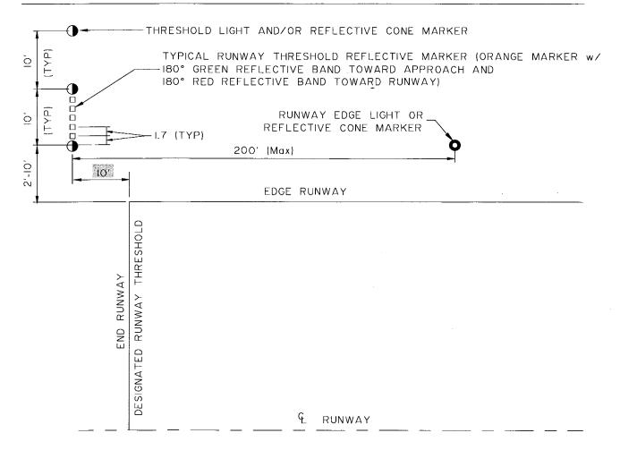
Figure 660-1 Typical Threshold Detail No Scale
