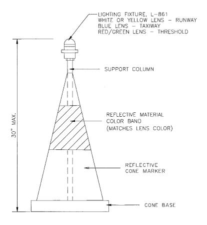
Figure 660-3 Reflective Cone Marker with Light No Scale
