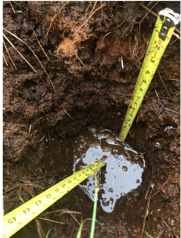
Figure 3: PD-4 Soil pit with water table rising (after approx. 15 minutes).
