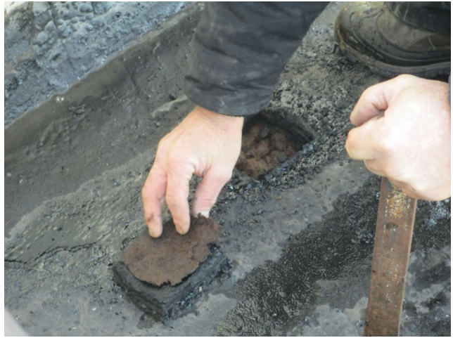
Photo 14: Wildwood Bldg 8 – Roof B @ Mechanical Room Core Cut #2 Disassembly
