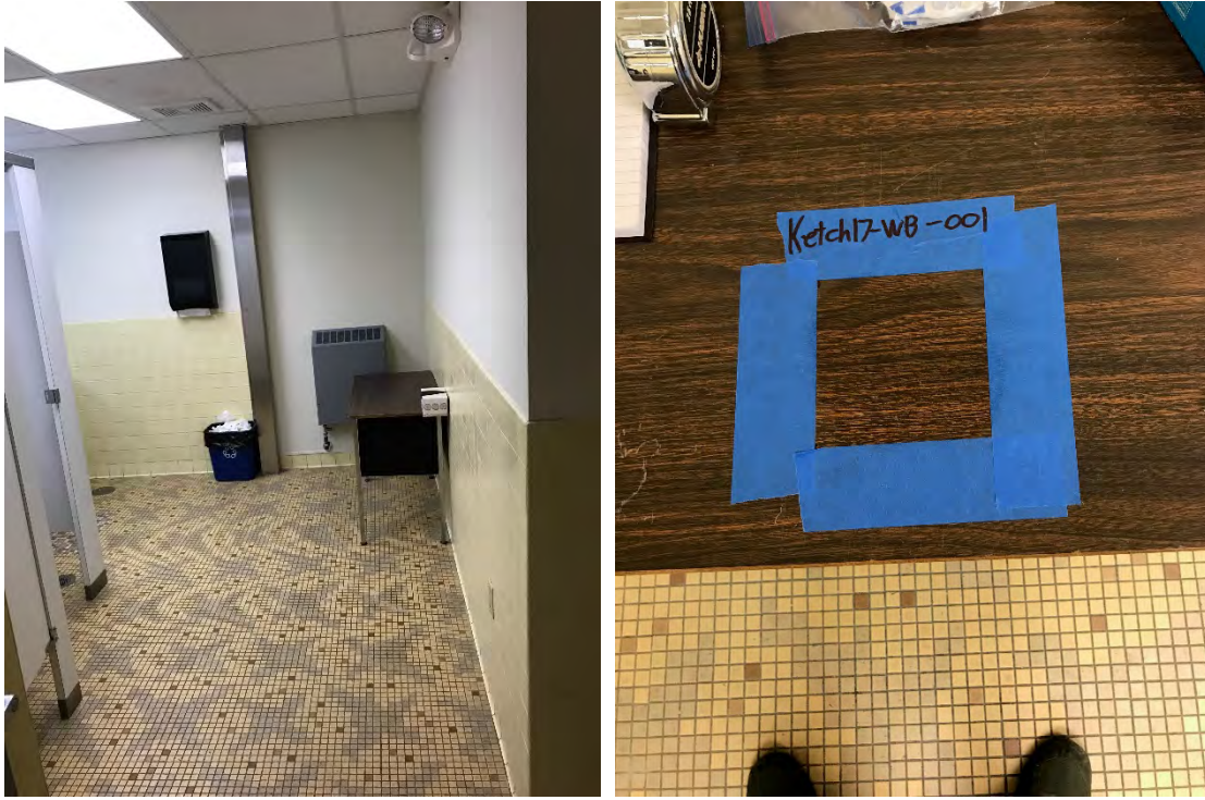
Photos 94 and 95: Women's bathroom (left) and lead wipe sample from surface of table in women's bathroom (right).
