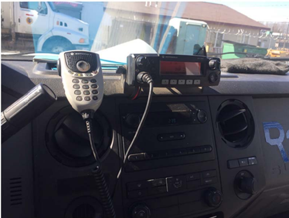
Photo 02: Example of remote head and hand mic mounting locations
