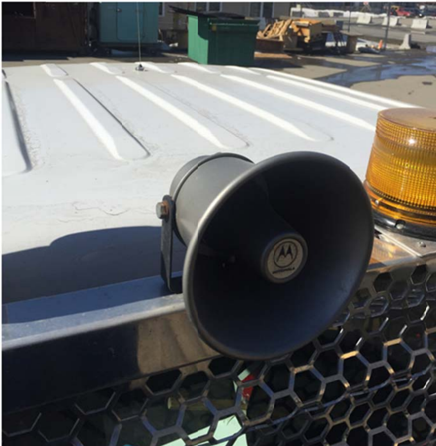
Photo 04: Example of external speaker and antenna mounting locations
