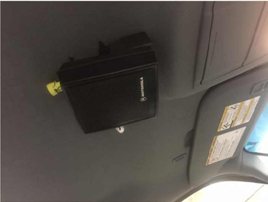
Photo 03: Example of internal speaker installation location
