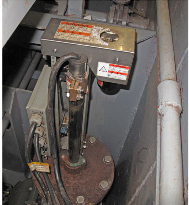
Figure 4.05B: Sonar Mounted on an 8 inch Sea Chest in the Tank Alley
