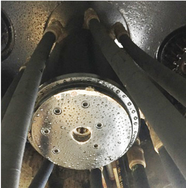
Figure 6-3: Hydraulic Hose Connections to Rotoseal at Base of Crane Turret.
