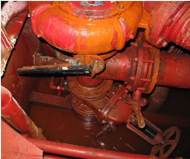
Figure 8-1: Port sea chest with 8 inch gate valve.
