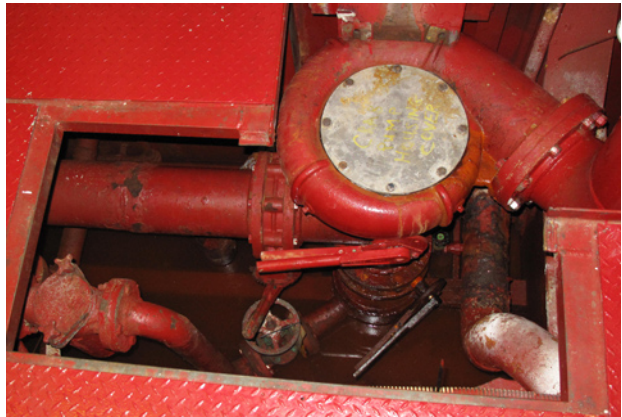
Figure 8-2: Starboard sea chest with 8 inch wafer sea valve and 3 inch fire pump suction.
