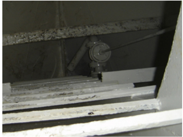
Figure 7-1: Forward Ballast Tank Valve and Reach Rod, Inside Forward Ballast Tank
