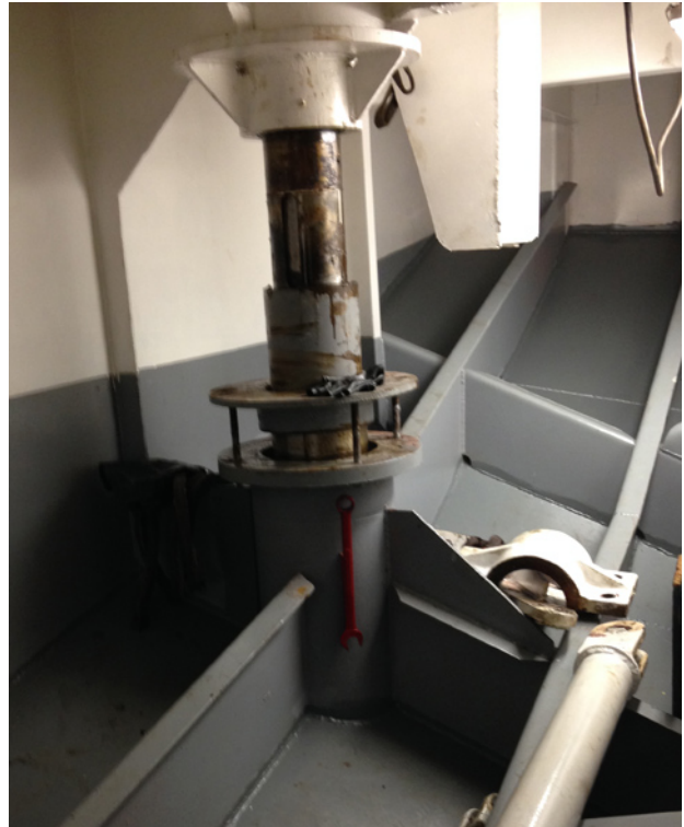
Figure 4.02A: Rudder Shaft in Lazarette with Tiller Arm Removed
