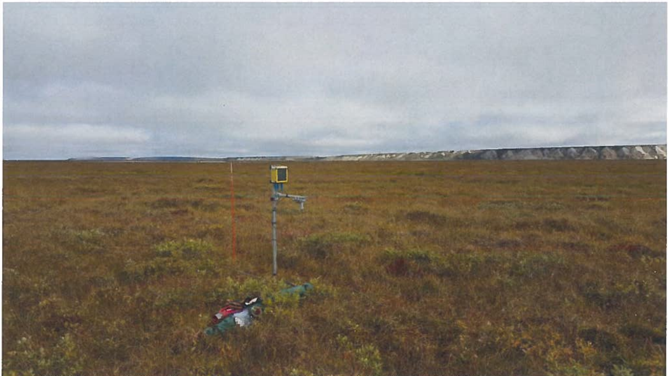
MP 1 Beaded Stream Data Logger looking northwest towards Franklin Bluffs. There are two ground sensors collecting data. The north sensor lead is the control "off-road" sensor. The south sensor lead will be the "on-road" sensor that will be used to track the pre-packed portion of the trail.
