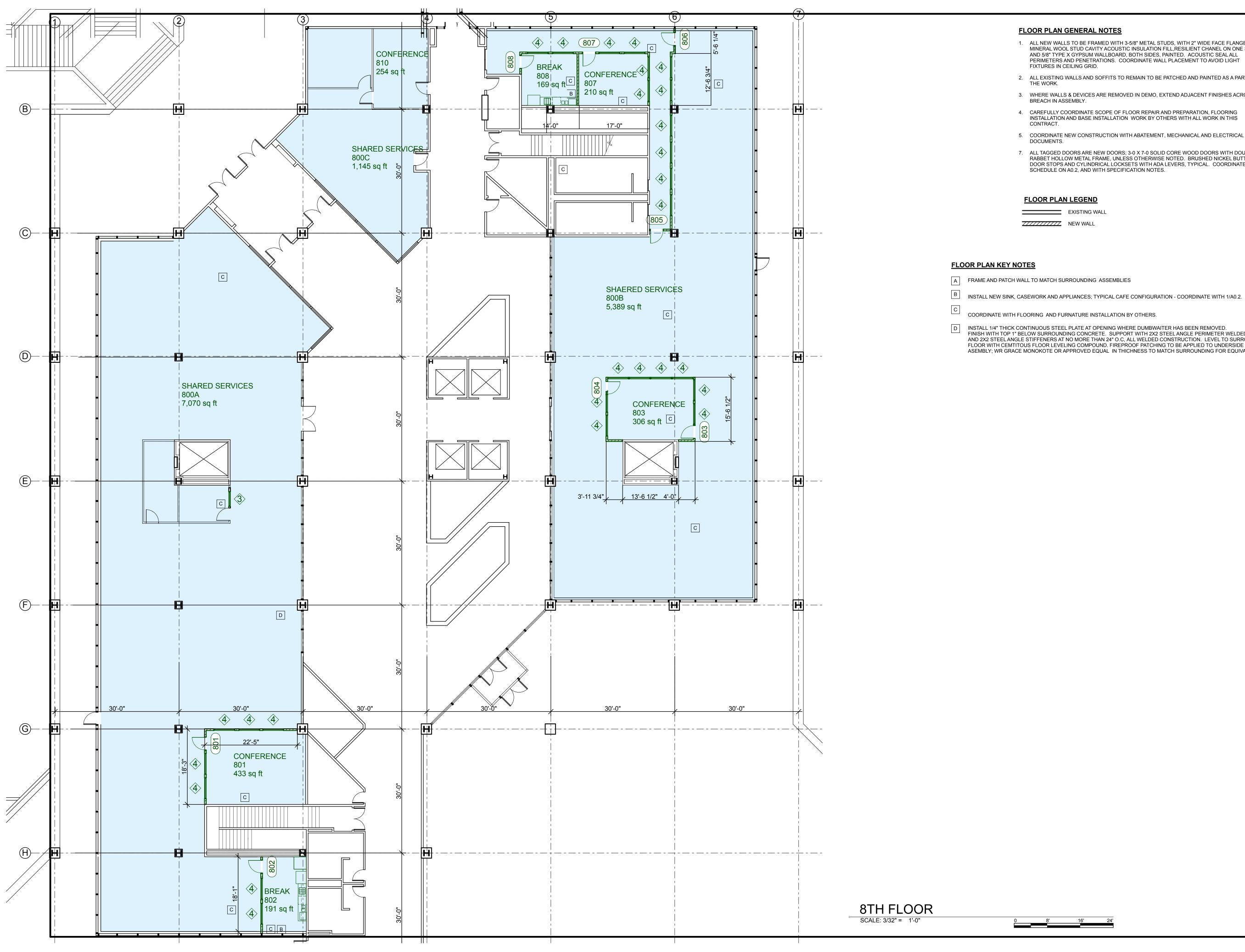
1. ALL NEW WALLS TO BE FRAMED WITH 3-5/8" METAL STUDS, WITH 2" WIDE FACE FLANGES, MINERAL WOOL STUD CAVITY ACOUSTIC INSULATION FILL, RESILIENT CHANEL ON ONE SIDE, AND 5/8" TYPE X GYPSUM WALLBOARD, BOTH SIDES, PAINTED. ACOUSTIC SEAL ALL PERIMETERS AND PENETRATIONS. COORDINATE WALL PLACEMENT TO AVOID LIGHT
