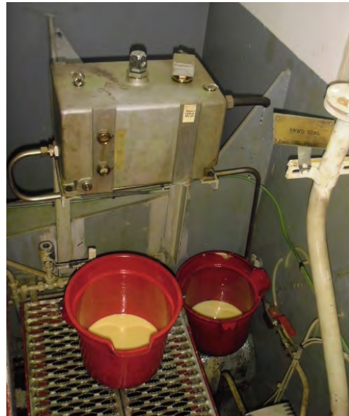
Figure 12-Example leak potential into bilge
