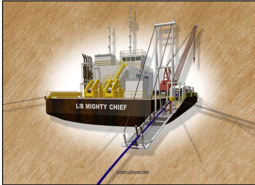
Photo 1: Example Lay Barge with Stinger
