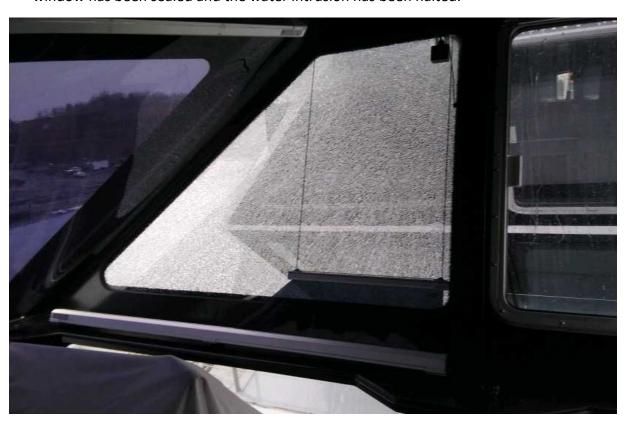
2. This picture is the FVF Fairweather Port Bridge area. While the window is intact, there is a tear or crack immediately above it and the wiper is smashed. There is water intrusion into the bridge area of the FVF Fairweather due to this damage. However, while tear or crack will not be repaired before the sale, the area has been sealed and the water intrusion has been halted.
