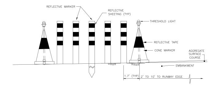
Figure 660-2 Threshold Reflective Marker Details No Scale
