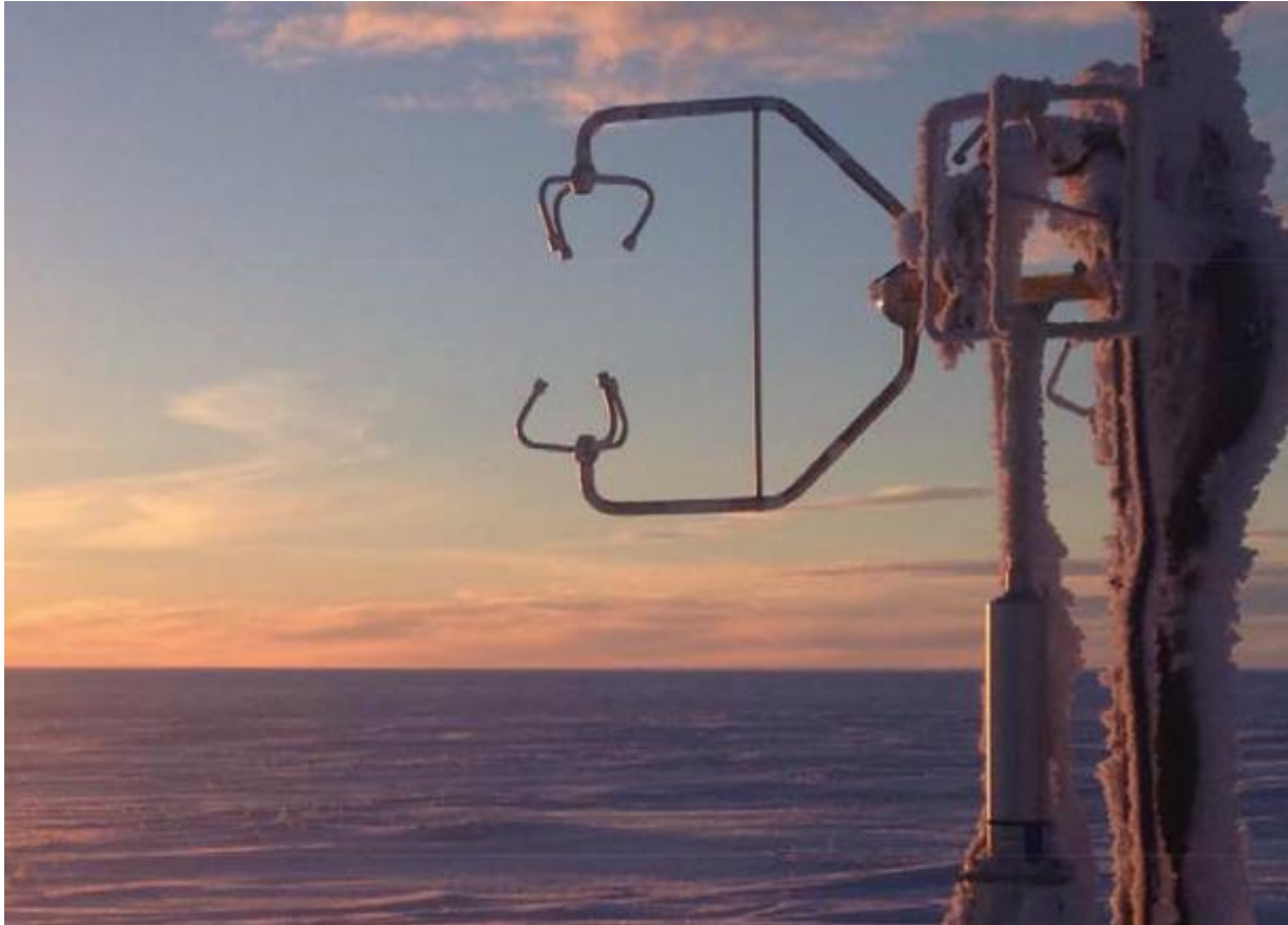
Fig. 4: Metek Heated Anemometer
