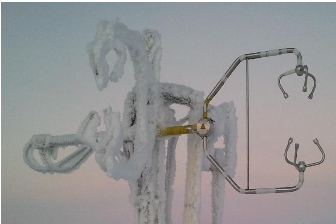
Fig. 5: Heated Anemometer (right) Compared to Regular Anemometer (left)
